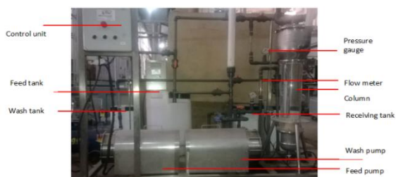
Fig. 1. Photo of pilot-scale adsorption system using the fluidized bed column
