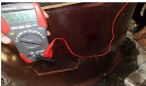
Fig. (20): Natural Tank/ Soil Potential Measuring at the Perimeter
