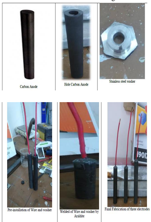
Fig. (9): Fabrication of three graphite electrodes.
