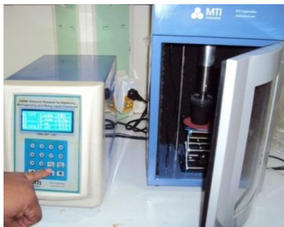
Fig. 1. sonication probe used for mixing process
