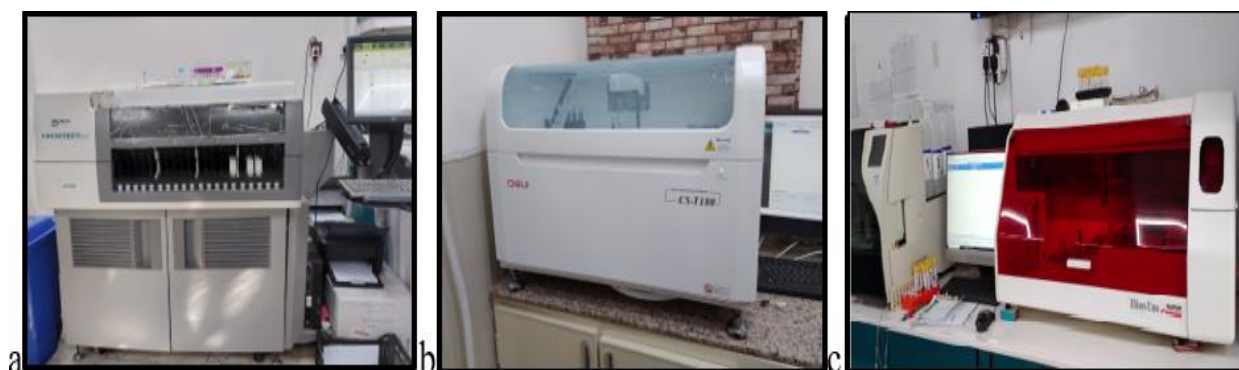
Figure 2: Photographs shows: (a) Abbott Architect c4000 clinical chemistry analyzer. (b) Fully automatic DIRUI, Auto-Chemistry Analyzer. (c) Elisys Uno, fully automated ELISA analyzer
