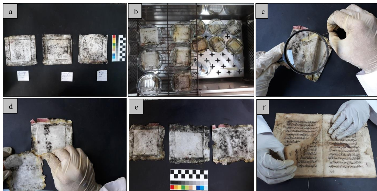
Fig. 4. Enzymatic disassembling of caked papers; (a) caked papers, (b) immersion in enzymatic solution and incubation at 40 °C, (c) and (d) disassembling of caked papers using needles with the help of magnifying lenses (e) Caked papers after separation and (f) Manuscript under investigation during separation.
