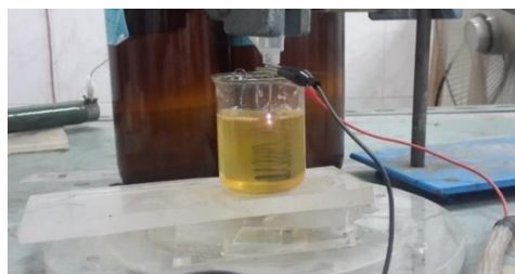
Figure 2: Photograph of glow discharge in contact with liquid
