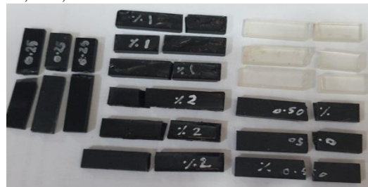
Fig.2. Pure epoxy and their nanocomposite samples were tested for each mass fraction of MWCNTs
