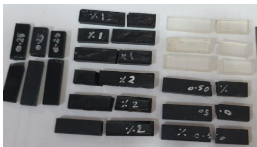
Fig.3. shows impact specimens after the test. Impact strength
