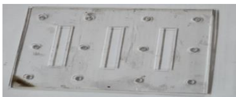
Fig.1. Molds of impact test by using a Computer Numerical Control (CNC)
