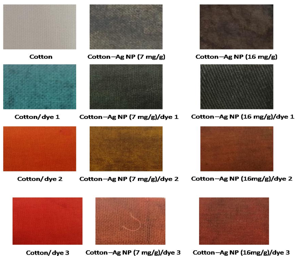
Figure 6: Images of untreated cotton fabric, dyed with Ag NPs with content of 7 mg/g or 16 mg/g and printed with three different reactive dyes
