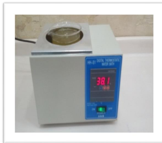
Fig (2) Picture of weight loss experiment with bulrush inhibitor.
