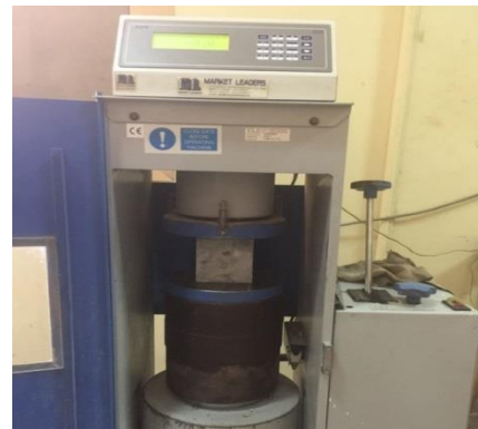
Figure 4. Compression test of concrete samples
