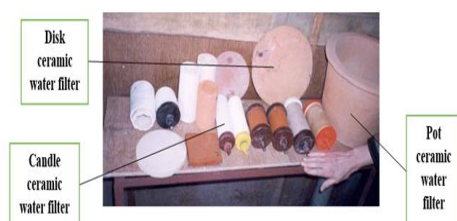
Fig. (9): Types of Ceramic Water Filter Elements according to its shape
