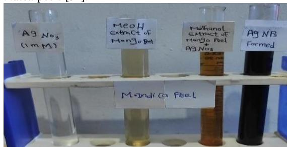
Fig. (5): Change in Color of the reaction mixture during formation of Ag NPs.
