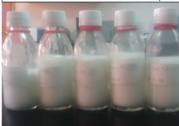
Fig.4. copper strips immersed in Metal cutting fluids.
