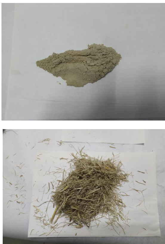
Fig. 1 Two bagasse samples: with milling, fine powder bagasse passed from mesh No 325 (left) and coarse bagasse fibre bundles without milling (right).
