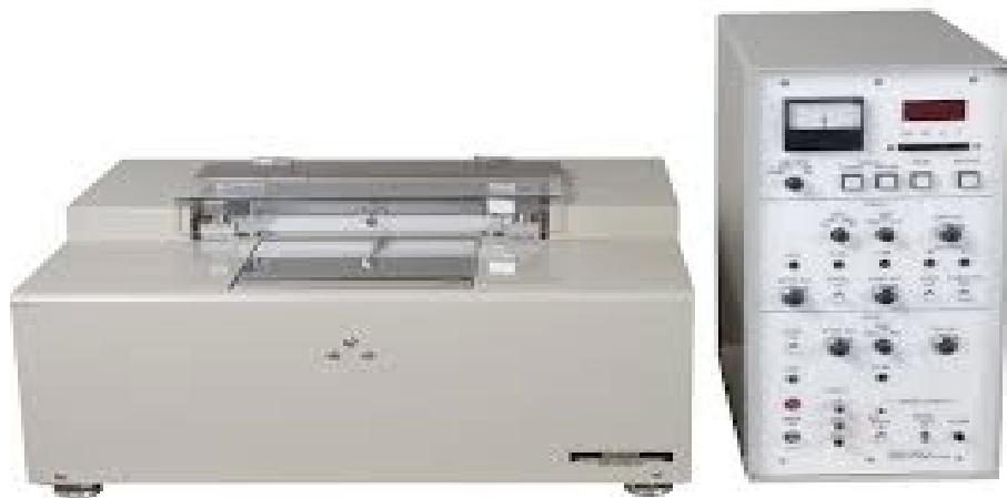
Fig. 1. Kawabata Evaluation; system KES-F (Tensile and Shear).
