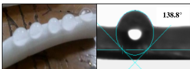
Figure 12: Water droplet on TBHF Composite membrane and its contact angle
