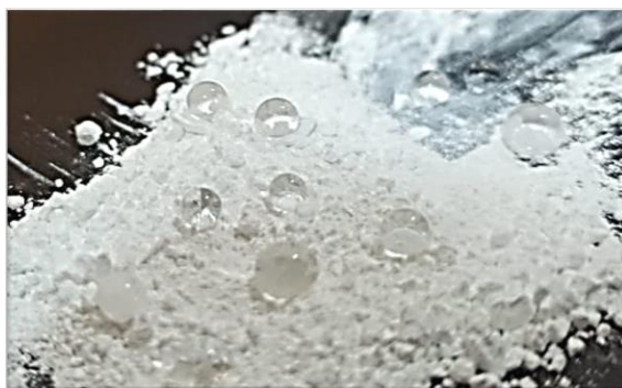
Figure 7: Digital photo of water droplet on FTiNPs particle
