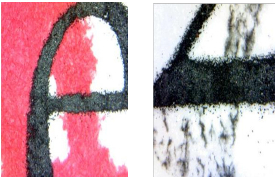
Fig. 6. The continuity gloss of toner and discontinuity ink gloss when (a) red Faber Castell and (b) black Horse inks are over a toner under a digital microscope.
