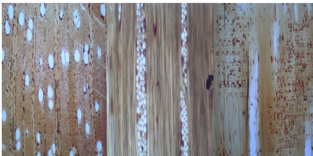
Figure 2: Light microscope images where a. Transverse section (TS); b. Tangential section (TLS); C. Radial section (RLS) of tamarisk wood ( Tamarix sp. L.) taken from statuette no. 1408
