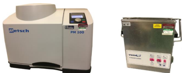
Figure 21: Typical laboratory employed planetary ball mill and ultrasonic bath
