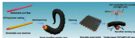
Figure 4. Schematic of the fabrication processes of carbon nanotube-incorporated nanofiber sensing yarn[34].
