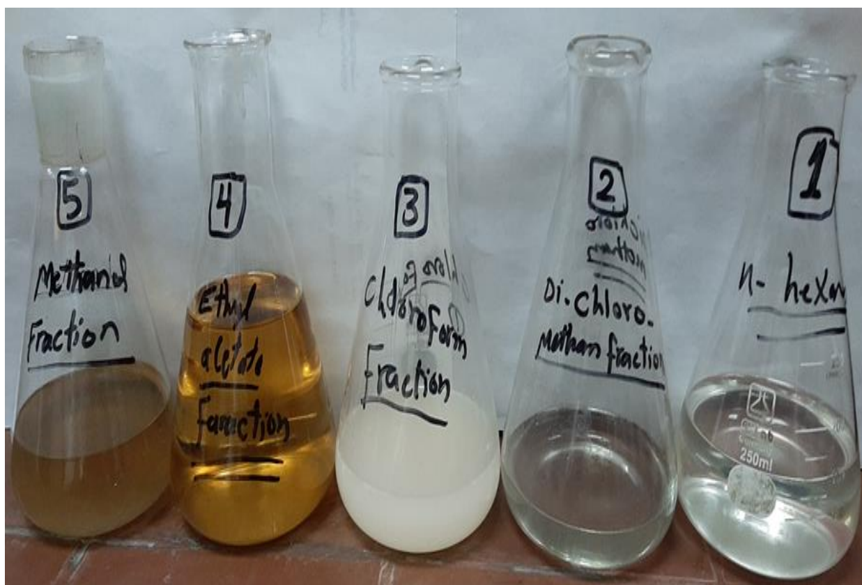
Figure (10): Successive extraction of the cell free MS fermentation broth with different solvents of different polarities.
