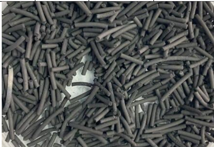
Fig.1. Granular activated carbon obtained from rice husk, oil sludge and polyvinyl acetate in a mass ratio of 9:1:1.1.
