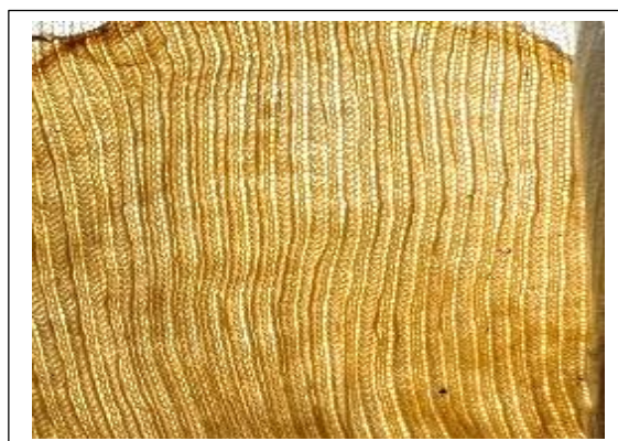
Fig. 2. Transparency after reinforcing with knitted fabrics from the back 'Source: Author's own creation'
