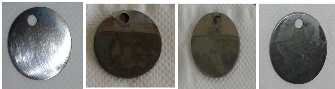
Fig. 9. Macrostructure of the mild steel for the blank sample and for investigated complexes [Cd(II) and \text{UO}_2(\text{II}) ]
