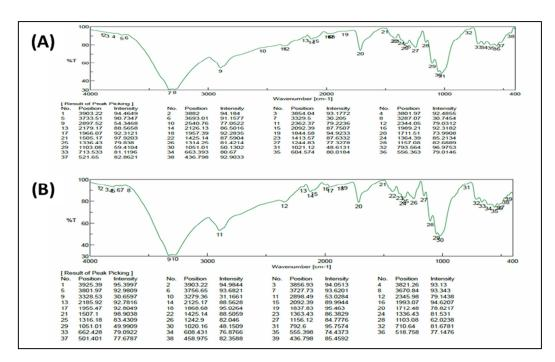
Figure 7: FT-IR Spectra of PET/C Blended Fabrics Waste Activated and Loaded with Biosynthesized NPs\*. (A)PET/C+E; (B)PET/C+E+CuO after Five Washing Cycles According to AATCC Test Method (61-1989) E=Cellulases
