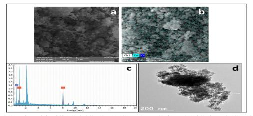
Figure 2: Some characteristics of *Chlorella*-CuO-NPs: Scanning electron microscopic micrographs (a & b), elemental analyses (c) and HRTEM micrographs (d)
