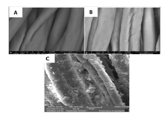
Figure 6: SEM Micrographs of Activated PET/C Blended Fabrics waste and Loaded with Biosynthesized NPs\* (1000x). (A) PET/C; (B) PET/C+E; (C) PET/C+E+ CuO. \*After Five Washing Cycles According to AATCC Test Method (61-1989). E=Cellulases
