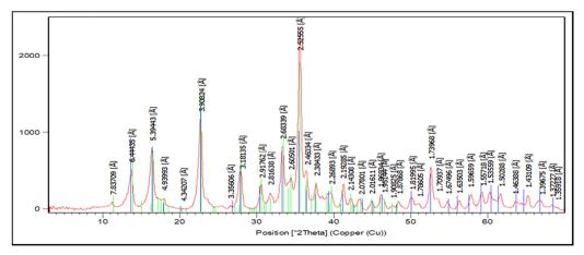
Figure 4: XRD pattern of microalgal synthesized CuO-NPs
