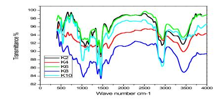
Fig. 2. FTIR spectra of polymer nanocomposite K2, K4, K6, K8 and K10.
