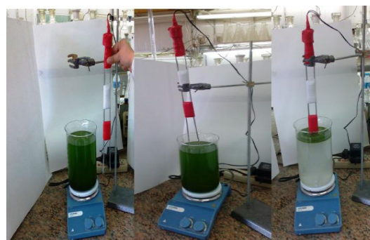
Figure. 1. Cultivation and harvesting of Dunaliella salina micro algae. (a) Cultivation of Dunaliella salina in open ponds. (b) Harvesting using electroflocculation.
