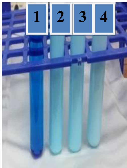
Fig. 7a. Decolorization of MB Dye in finishing formulations contain TiO 2 nanoparticles in presence of different concentrations of cationic softener concentrations where (1) 20mg/L MB (2) 10 ml of 20mg/L MB with 40 ml of ( 2% huntsman Cationic softener/1% Ti nano ) (3) 10 ml of 20mg/L MB with 40 ml of ( 3% huntsman Cationic softener/1% Ti nano ) (4) 10 ml of 20mg/L MB with 40 ml of ( 5% huntsman Cationic softener/1% Ti nano).
