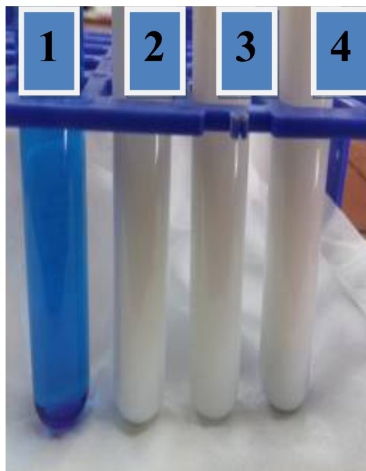
Fig. 7a. Decolorization of MB Dye in finishing formulations contain TiO 2 nanoparticles in presence of different concentrations of cationic softener concentrations where (1) 20mg/L MB (2) 10 ml of 20mg/L MB with 40 ml of ( 2% huntsman Cationic softener/1% Ti nano ) (3) 10 ml of 20mg/L MB with 40 ml of ( 3% huntsman Cationic softener/1% Ti nano ) (4) 10 ml of 20mg/L MB with 40 ml of ( 5% huntsman Cationic softener/1% Ti nano).
