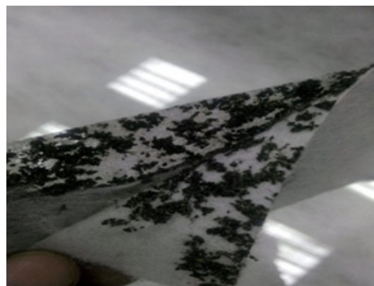
Fig. 2. Nonwoven fabric containing activated carbon
