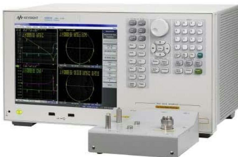
Fig. 2.2.1. The wide range frequencies between 1 MHz and 1 GHz using network impedance analyzer (KEYSIGHT-E4991B).
